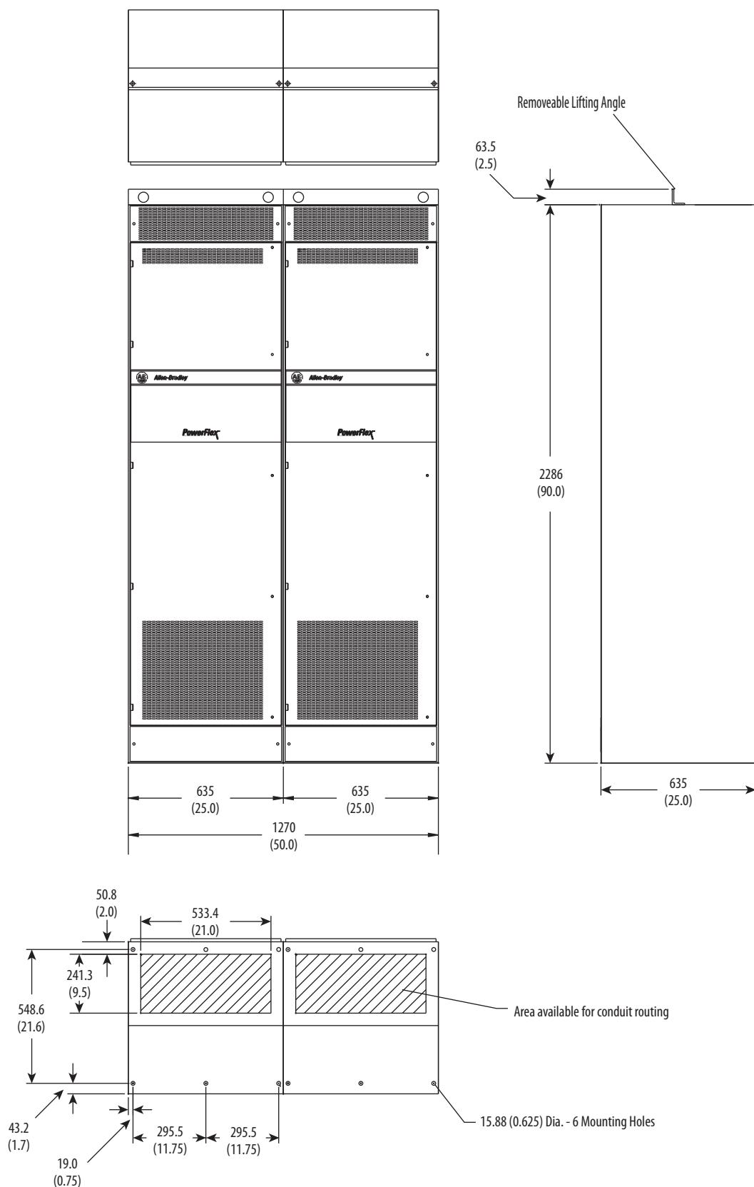
**Frame 12, NEMA/UL Type 12, IP54 (Enclosure Code "H")**
