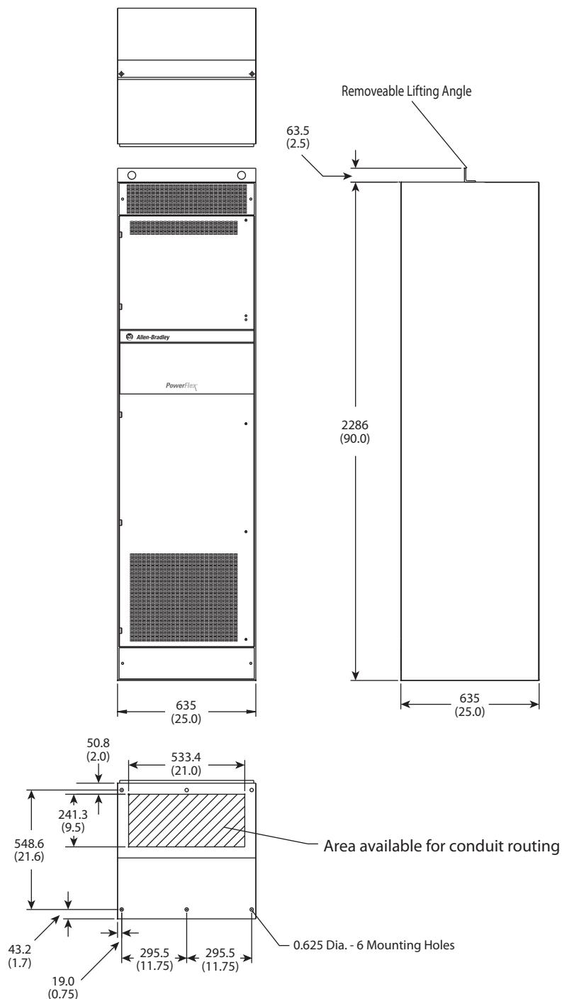
**Frame 10, NEMA/UL Type 12, IP54 (Enclosure Code "H")**
