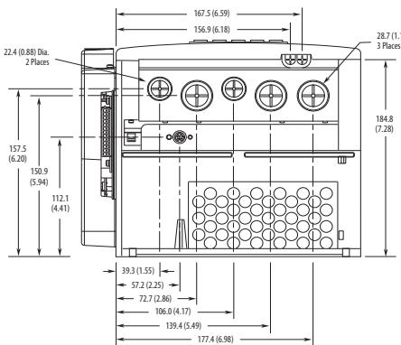
Frame 3 - All Drives except 50 HP, 480V (37 kW, 400V) Normal Duty Drive
